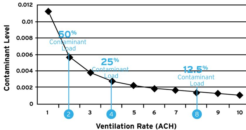
Figure 6 Impact of Air Changes per Hour (ACH) on viral load<sup>26</sup>
