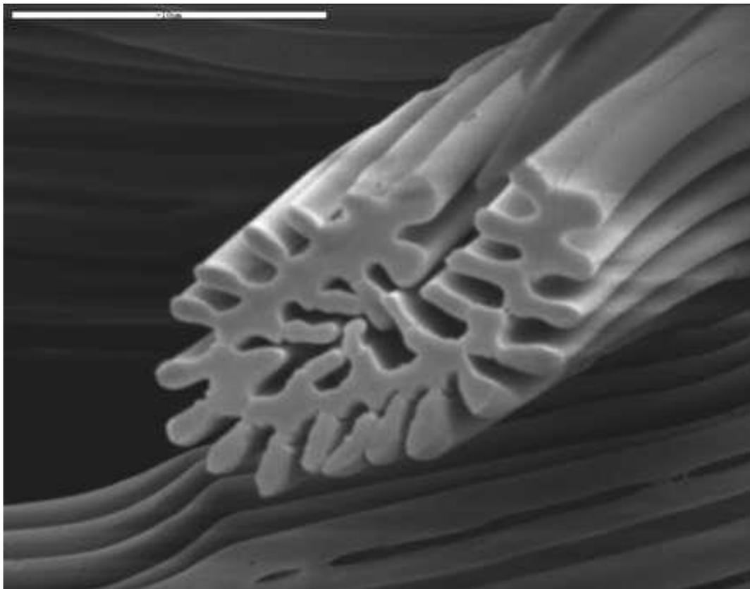
*Figure 8 Scanning Electron Microscope image of a Winged Fiber<sup>32</sup>*
