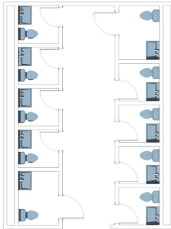
*Figure 16 Bathroom design with individual washrooms to limit exposure to a single area.*
